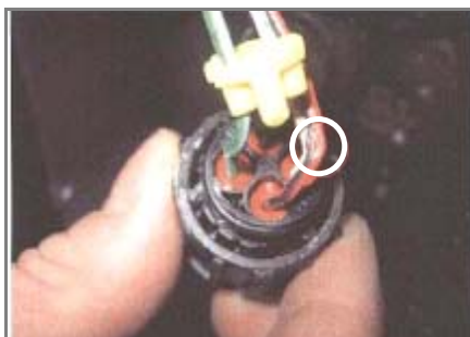
Damaged wires
